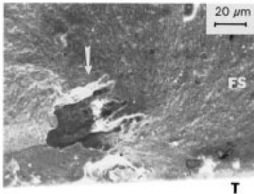
**MATERIAL:** Sintered Yttria-tetragonal zirconia polycrystal, as-machined
