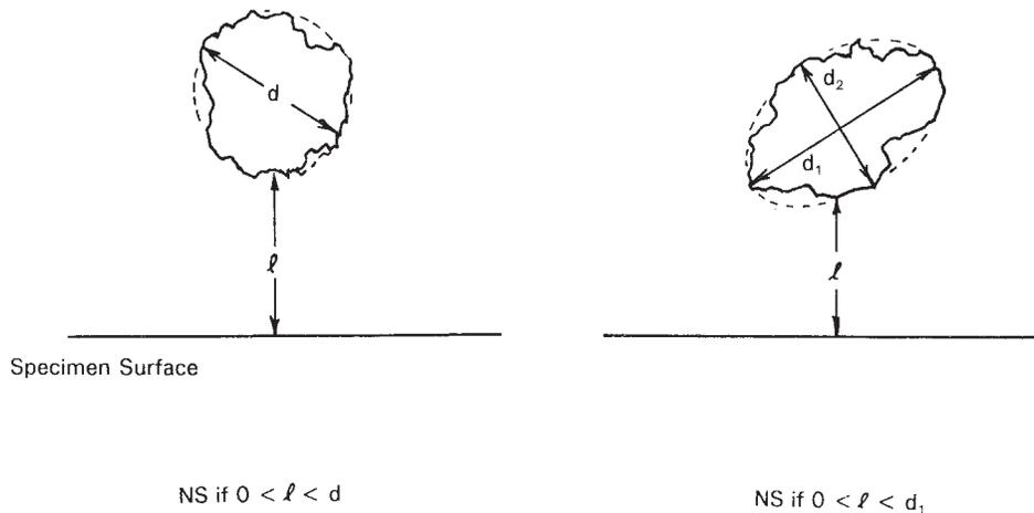
NOTE 1—Origins can be characterized as near-surface (NS) depending upon whether they are within the distances illustrated. The origin size is the diameter for equiaxed origins, and is the length of the minor and major axes of an elongated origin. All measurements dimensions are approximate only.
