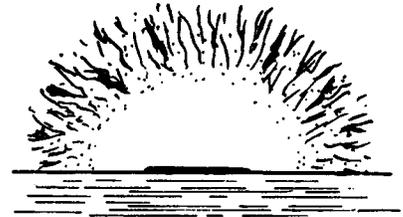
(b) **elongated “coplanar parallel crack”** linked with a **natural flaw**. A step in the fracture origin emanates from the discontinuity.
