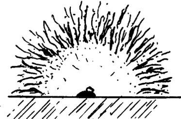
(d) shows the same as above, except that the natural flaw created a bump or jog in the fracture mirror. The irregularity at the origin created a step or curve in the fracture mirror that created a tail that extends well up into the mirror or even to its boundary.
