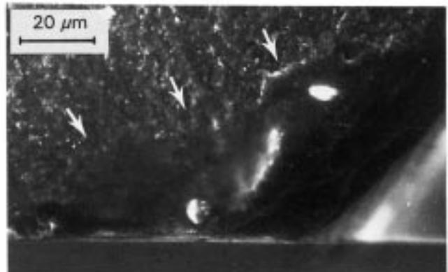
NOTE 1—Masking tape is sometimes used to hold pieces of a fractured specimen together, but should be avoided on the fracture and tensile surfaces. The smear blends into the fracture surface and is partially transparent to X rays as shown. An energy dispersive analysis identified the smear as having potassium, chlorine, and sulfur. Trichloroethylene is an effective solvent to remove the resin.
