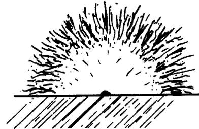
(c) shows a machining crack that linked up with a natural material flaw such as an agglomerate or pore. The origin may be categorized either as an enlarged natural flaw or a hybrid natural flaw-machining damage. The natural flaw may make the material more susceptible to machining crack damage in the immediate vicinity of the flaw than elsewhere.
