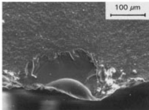
**MATERIAL:** Hot-pressed Silicon Nitride with Magnesia additions, as-machined
