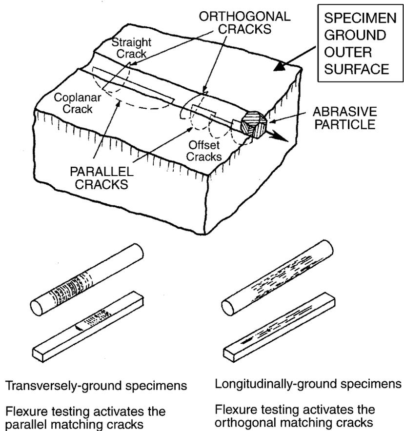
NOTE 1—The machining cracks extend much deeper into the bulk than the striation-grooves on the surface.
