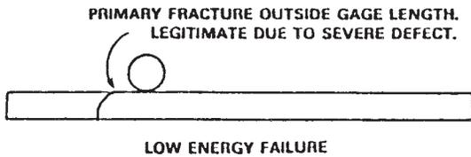
FIG. X6.1 Typical Fracture and Crack Patterns of Flexure Specimens
