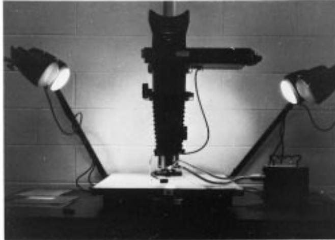
FIG. X4.5 Macrophotographic Camera Stand for Instant Photographs
