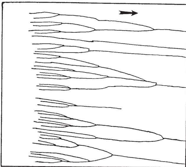
NOTE 1—The direction of crack propagation is shown by the arrow.
