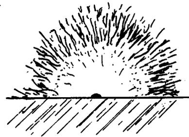
(b) shows the same as above, except that an unusually deep machining striation is lined up with the machining crack. Deep striations may aid interpretation, but they may not necessarily be present since final finishing may eliminate any such traces.
