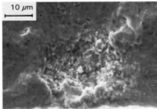
**MATERIAL:** Sintered Yttria-Tetragonal Zirconia Polycrystal, as-machined
