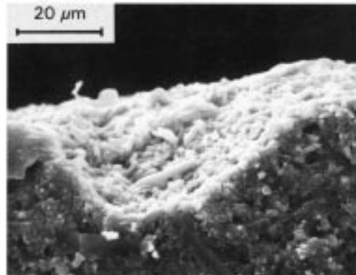
**MATERIAL:** Injection Molded & HIP'ed without a cladding, Silicon Nitride with Yttria & Alumina additions, as-fired
