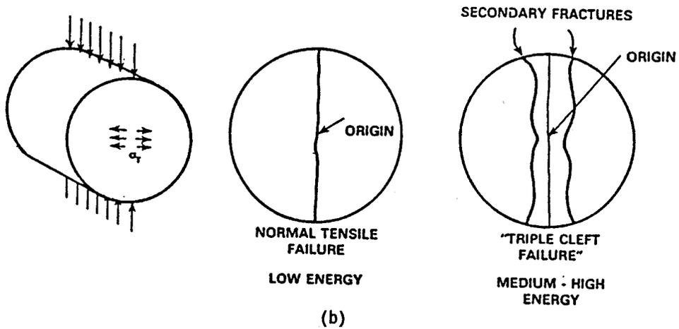
FIG. X6.2 Typical Fracture and Crack Patterns of: (a) Biaxial Flexure Specimens and (b) Diametral Compression Specimens
