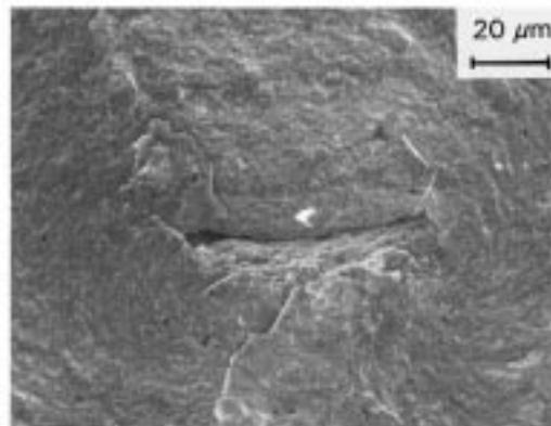
**MATERIAL:** Not isostatically pressed Yttria-Tetragonal Zirconia Material, as-machined
