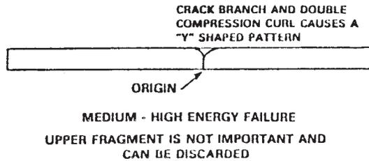
A SECONDARY FRACTURE CAUSED BY THE ELASTIC RELEASE WAVE - REFLECTION OFF OF THE END FACES. NOTE THIS OFTEN OCCURS AT LOAD PINS. NOTE THE MIRROR IS ON WHAT ORIGINALLY WAS THE COMPRESSION SIDE.
