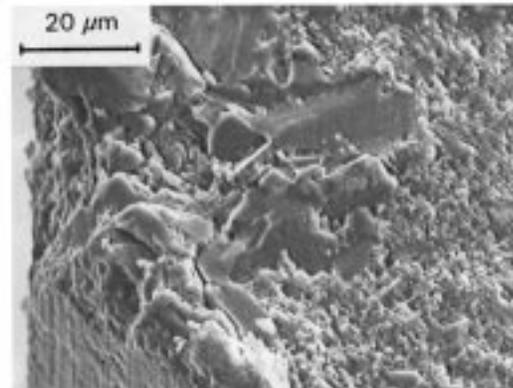
**MATERIAL:** Sintered (99.9% pure) Alumina, as-machined
