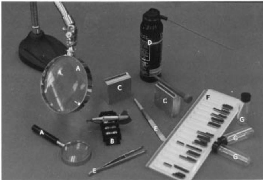
NOTE 1—(A) Hand-held and tabletop magnifying glass; (B) Variable-angle grips with compliant surface; (C) Fixtures to support specimens to view machined surfaces; (D) Compressed air; (E) Tweezers for specimen manipulation; (F) Plastic storage trays; (G) Glass vials for storage of fractured specimens prior to SEM analysis.
