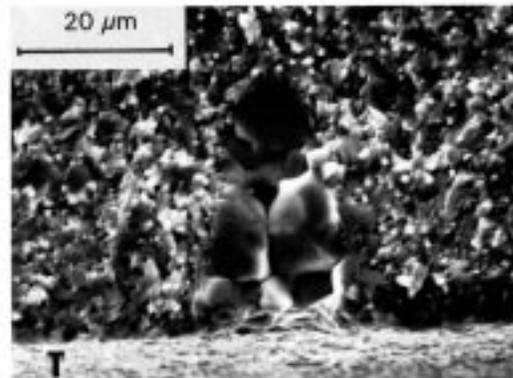
**MATERIAL:** Hot-pressed Alumina reinforced with Silicon Carbide whiskers, as-machined
