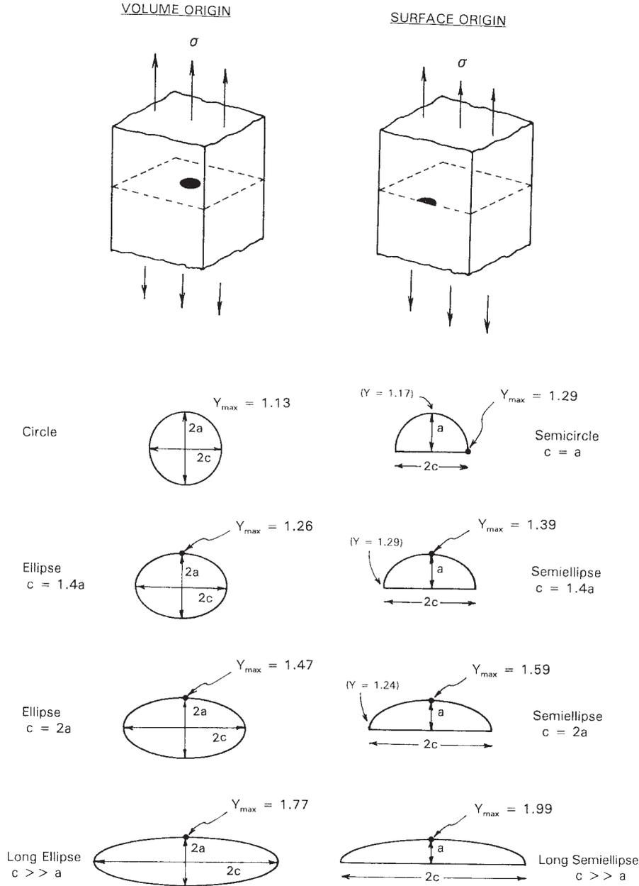
NOTE 1— $Y_{max}$  is shown for each example. The  $Y$  at the other points of the crack periphery is shown (in parentheses) for comparison in a few examples.
