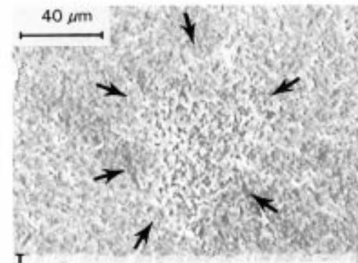
**MATERIAL:** Sintered SiAlON with Yttria & Alumina additions, as-machined
