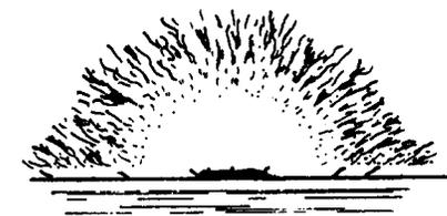
FIG. X9.3 Fractographic Signs of Machining Damage or Scratches
