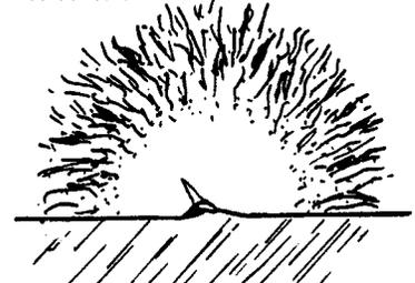
FIG. X9.2 Fractographic Signs of Machining Damage or Scratches
