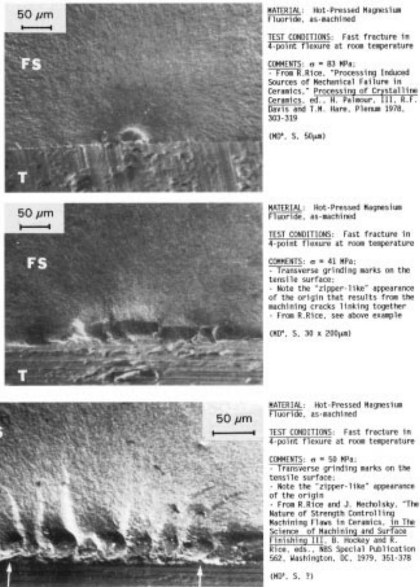
FIG. X1.10 Examples of Machining Damage (See Fig. X1.9)
