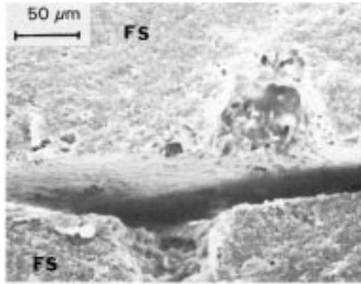
**MATERIAL:** Injection Molded & Sintered Silicon Nitride with Yttria & Alumina additions, as-fired
