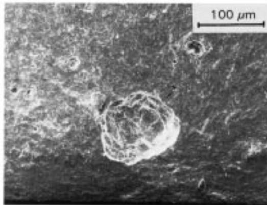
**MATERIAL:** Sintered Yttria-tetragonal zirconia polycrystal, as-machined
