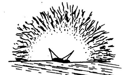
(f) **“coarse grinding parallel crack”**
