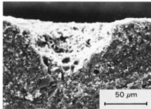
**MATERIAL:** Injection Molded & Sintered Silicon Nitride with Yttria & Alumina additions, as-fired
