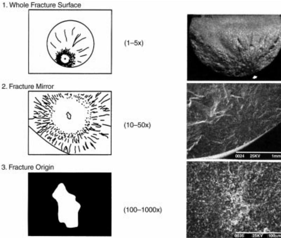
NOTE 1—(b) shows a sintered reaction bonded silicon nitride rod flexural strength specimen that had an inclusion origin  $\sigma = 751$  MPa maximum, 684 MPa at the origin center.
