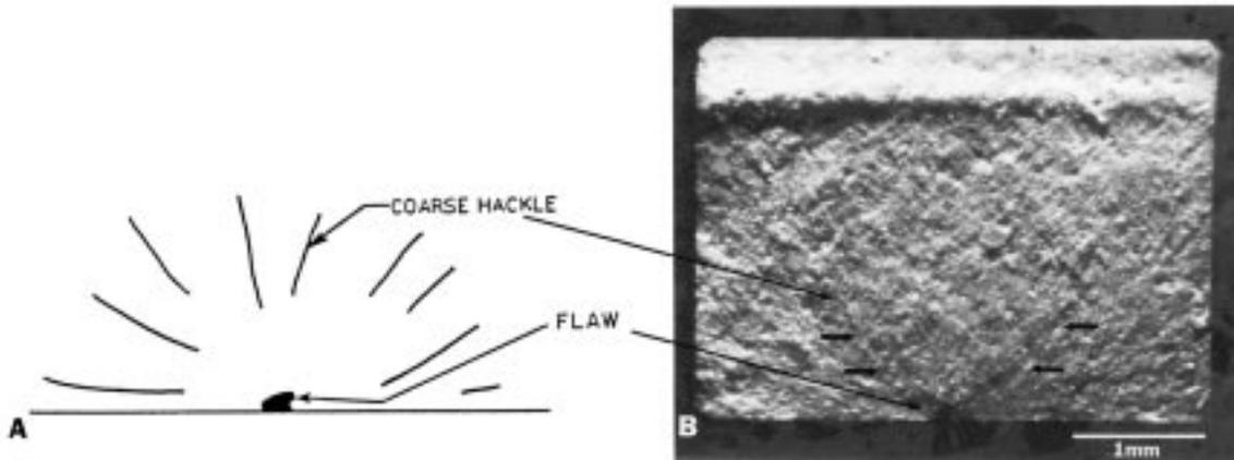
NOTE 1—The coarse hackle lines that emanate from the flaw can be used to locate the origin.
